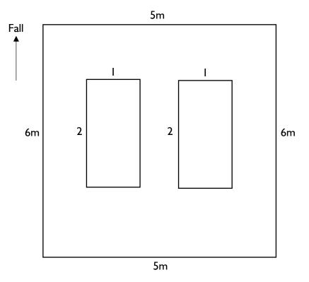
Area 30m2 take away 4m2 for roof lights. 26m2 of green area needed. To remove the area needed for pebble border and allowing for wastage multiple the area of the roof by 0.93 and round up the figure.
